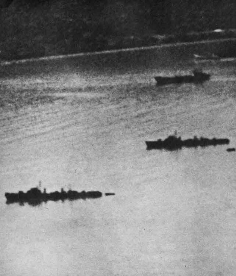
A low, simple profile characterizes Matsu Class, small DD's built in quantity for second-line duty. The second stack is abaft midships.
